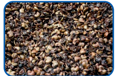
Cashew Shell Waste GROSS CALORIFIC VALUE (GCV) Kcal/kg: 5000+
