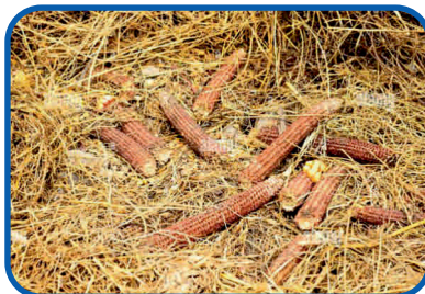
CORN COBS WASTE GROSS CALORIFIC VALUE (GCV) Kcal/kg: 3600-3800
