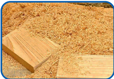
SAW DUST (WOODEN DUST) GROSS CALORIFIC VALUE (GCV) Kcal/kg: 4000-5000
